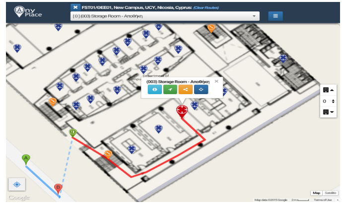
Fig. 5. The AnyPlace Indoor Information Service (screenshot relates only to the Web Viewer) facilitates the task of crowdsourcing models, context and radiomaps for indoor spaces but also supports intelligent search and navigation in buildings uploaded publicly or privately.
